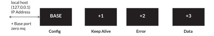
Each sensor on the Matrix has a mapped zero mq port with subports indicated above.
