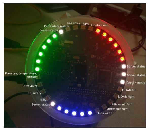
The LED ring (called Everloop) on the Matrix also serve as a dashboard/visual cue that data is being collected and all the sensors are operational. This is extremely important as most teams faced a problem where they thought the sensors were collecting data while testing but they weren't, either due to some error or that they weren't initialized properly.
