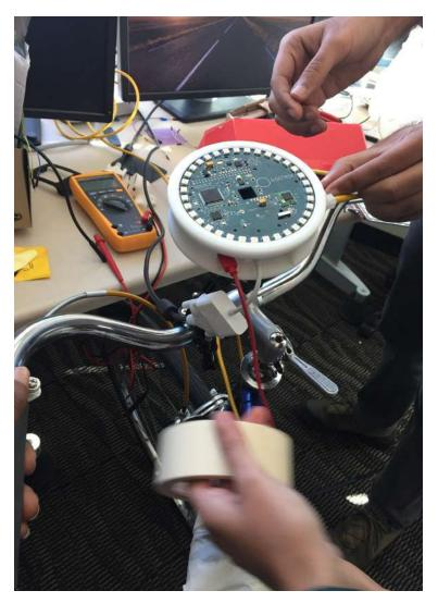
The matrix one is designed to work with a Raspberry Pi. It consists of multiple sensors including a 3D accelerometer, 3D gyroscope, 3D magnetometer, humidity sensor, temperature sensor, ultraviolet sensor, pressure sensors and more.
