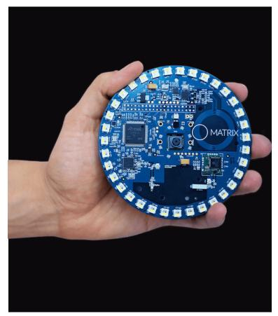
Matrix One Creator Edition (\$99) Raspberry Pi 3 (\$35) Anker 26800 mAh portable power bank Knowles BU21771 contact microphone GPS chip (in collaboration with the air quality team) 3D Printed Casing
